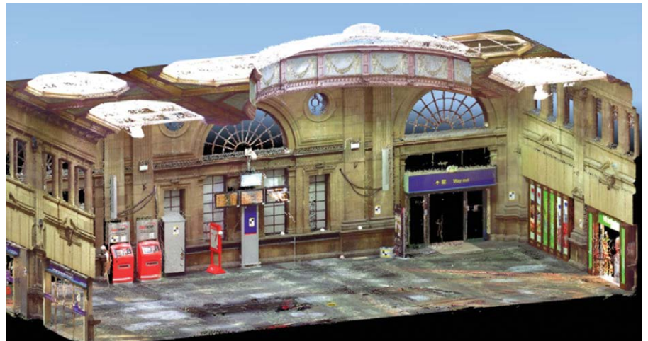
Figure 7 Waverley Station: Section view through the laser scan Point Cloud (Source: Historic England, 2017)
