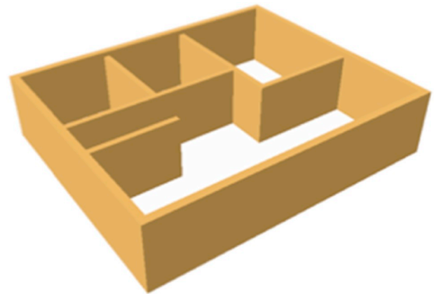
Fig. 18. Basic walls ( Wall_1 ) modeled using swept solid.
