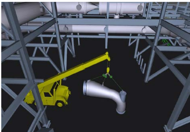
Figure 5: Screenshot of the 4D BIM Simulation on the System Level
