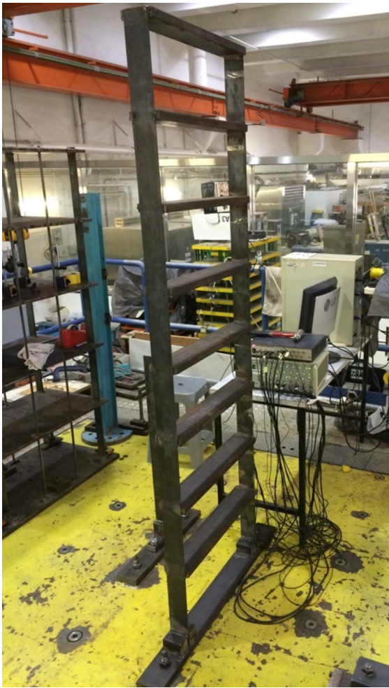
Fig. 12. Laboratory steel frame model.
