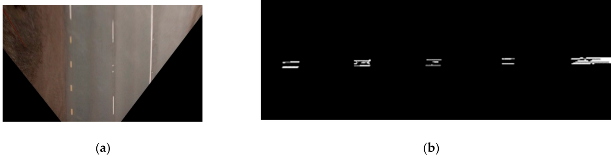
Figure 12. Example frame of false worn condition. (a) Planar image; (b) binary feature map of the yellow line marking.
