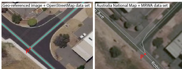
Figure 2. The picture on the left side shows a high-quality geo-referenced image with a data set of OSM, while the right image represents a National Map data set of the same junction with data from MRWA. The road connection points are indicated as 'P' (sources: http://spookfish.com (image left); http://openstreetmap.org (road data left); http://nationalmap.gov.au (image and road data right)).
