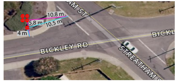
Figure 4. The illustration shows multiple data sets, as well as synthetic data (the group of four STOP signs) plotted on a geo-referenced image (sources: http://data.wa.gov.au (data); https://www.spookfish.com (image)).
