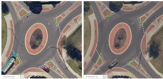
Figure 7. The left image shows a high-resolution satellite image from the 5 th September 2017, and the right image shows the same road asset section with data from the 18 th September 2017 (source: https://www.spookfish.com ). The green rectangles indicate the location of placed GIVE WAY signs.
