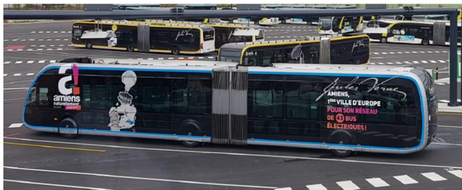
Figure 1: Trackless tram example (fully electric Irizar ie tram used on the Amentis Network for Amiens Metropole France operated by Keolis (Photo credits: Marie Verschuer)
