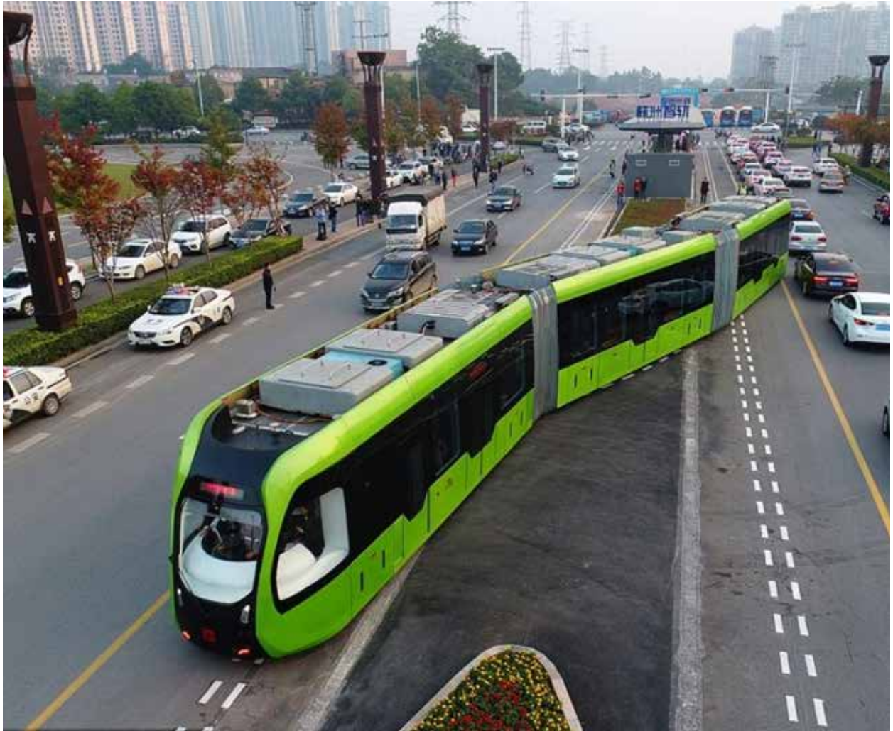
Figure 19. Autonomous Rail Rapid Transit in China showing electric battery-powered and autonomous guidance system. Source: CRRC Zhuzhou Institute
