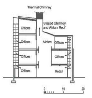
Figure 2: Ventilation strategy, showing thermal chimney<sup>27</sup>
