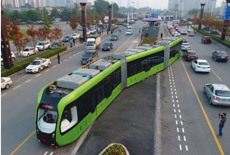
Fig. 3.3 The trackless tram system by CRRC and demonstrated in Zhuzhou, China. Source: Compliments of CRRC
