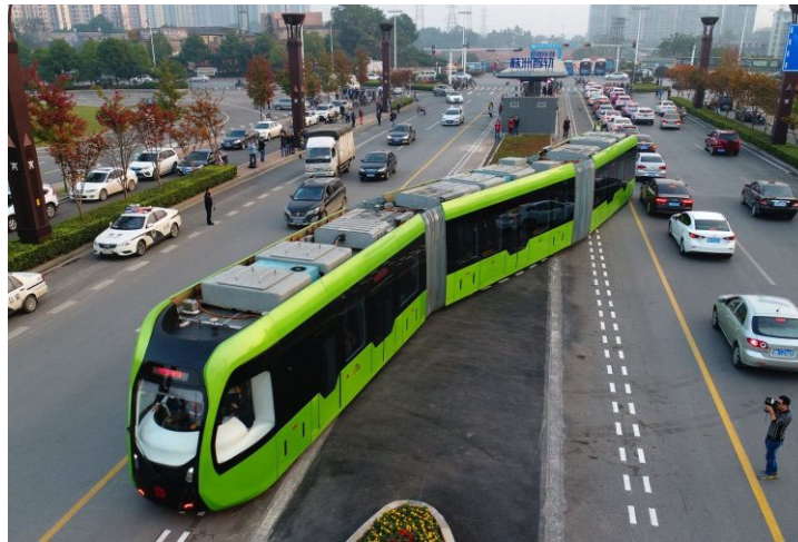
Figure 6. The new electric Trackless Tram in China showing its tram-like quality with modern sensors that enable its rail-like ride quality. Source: CRRC.
