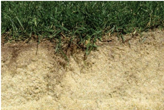
Figure 5. A cross-section showing established grass turf grown on a glass sand medium
