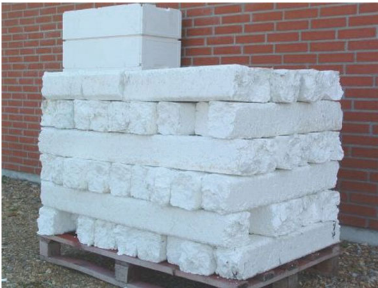
Fig. 2.6 Bars of EPS produced with densifier equipment. Source: https://tagliabrasil.com.br/com-pactadores-de-eps
