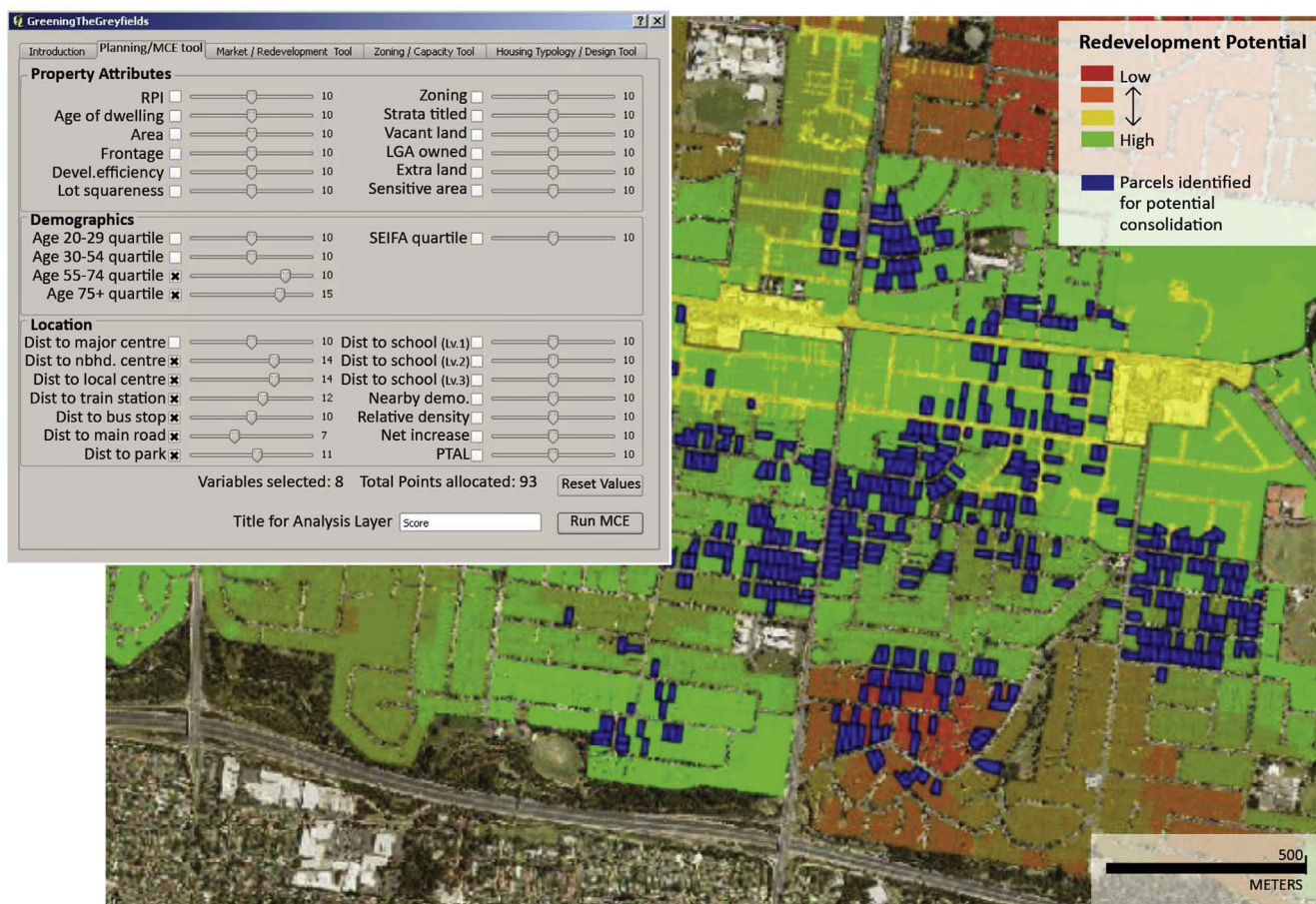
Fig. 4. ENVISION's Multi-Criteria Evaluation (MCE) input enables the user to select variables and weight their significance; Based on these criteria, ENVISION then selects land with highest redevelopment potential (green) and identifies parcels that could be consolidated for larger-scale development (blue) (Glackin, 2012). (For interpretation of the references to colour in this figure legend, the reader is referred to the web version of this article.)
